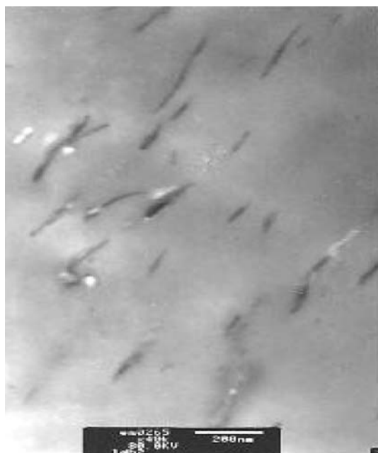
Fig. 4 TEM micrograph of PVDF nanocomposite having 3.85 wt.% LDH-DS (scale bar 200 nm)
